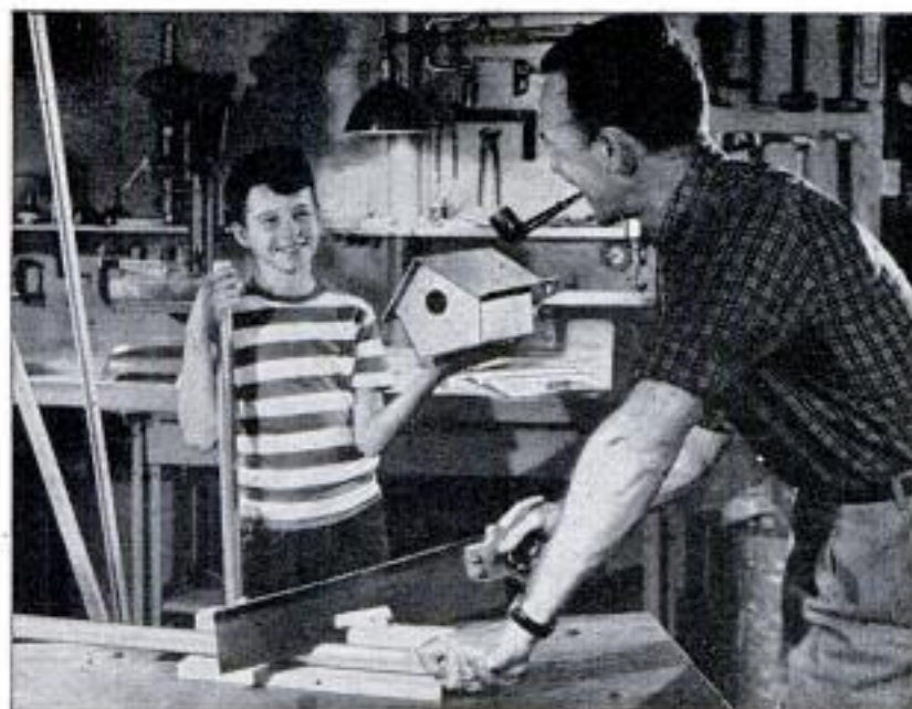
Wood Saws are fine for cutting Reynolds Do-It-Yourself Aluminum. Generally saws with a greater number of teeth per inch will cut more evenly and cleanly.
